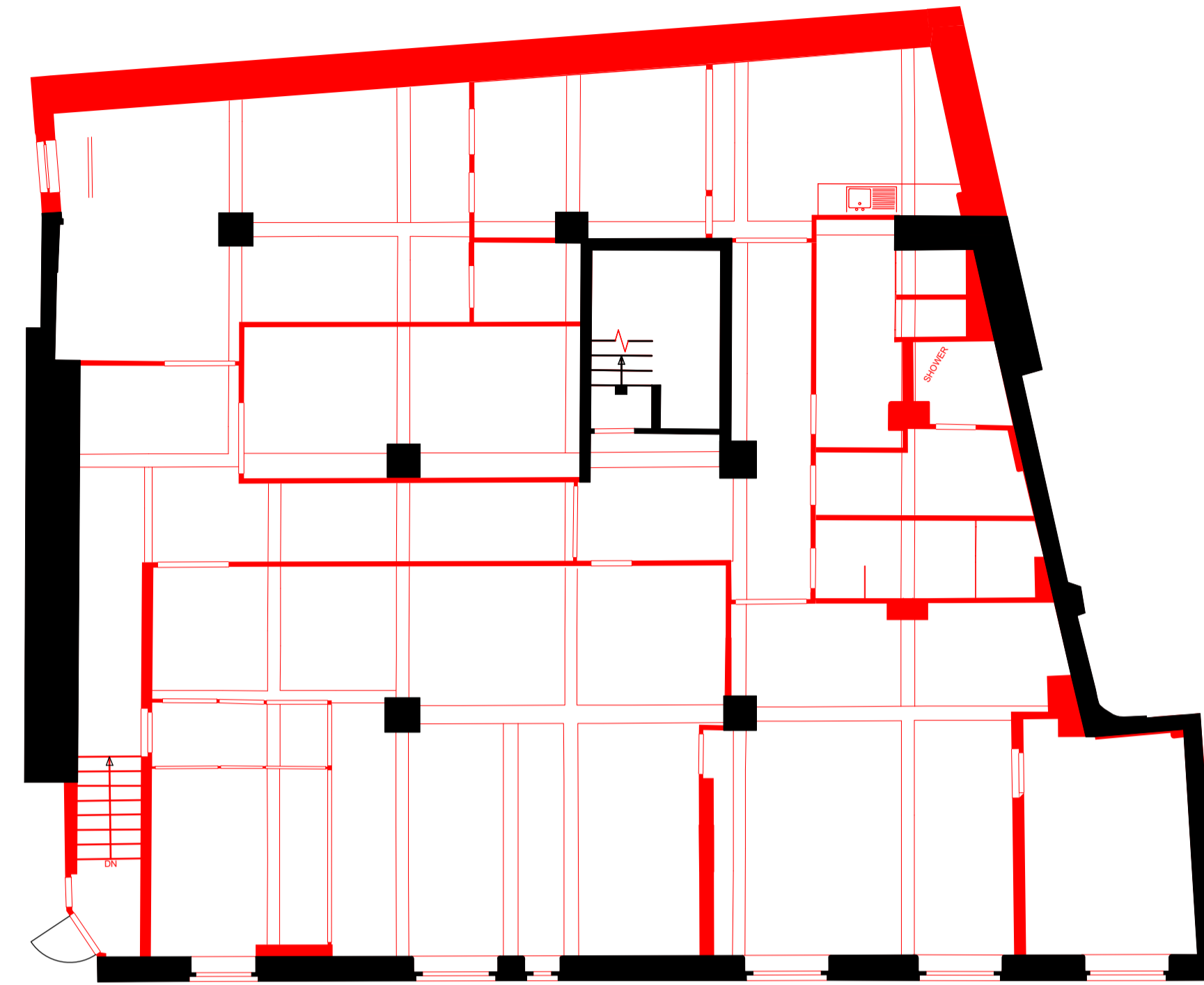
BASEMENT DEMOLITION PLAN 1:100 @ A1
