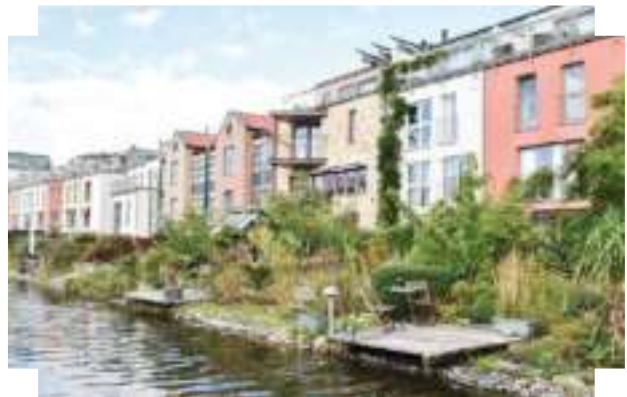
A visually interesting elevation, providing variety in material, roofscape. Upper storeys are recessed to create roof terraces | Malmo, Sweden
