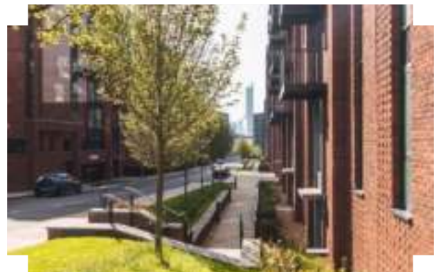
A combination of steps at the top of the slope and a level route at the lower level provides access to the building for people with different levels of mobility Middlewood Locks, Salford
