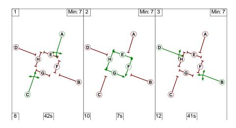
Phases A, B, C, and D represent the vehicle phases. Phases E, F, G, and H represent cycle phases.
