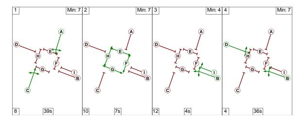
Phases A, B, C, and D represent the vehicle phases. Phases E, F, G, and H represent controlled pedestrian crossings phases. Phase I represents the proposed early right-turn indicative arrow phase.
