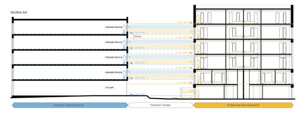
It is proposed that through careful placement and the orientation of windows, along with the use of louvres on the windows in this elevation, this would help to mitigate any direct overlooking further.
