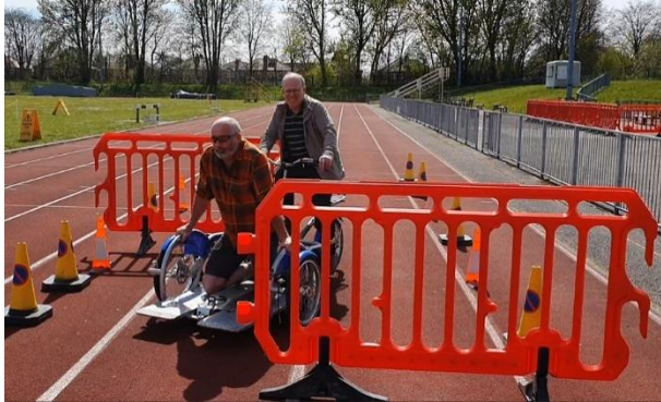
3.5m spacing chicanes on a 3m wide path with 0.3m overlap to reduce gap to 1.2m picture shows tricycle wheelchair tandem.
