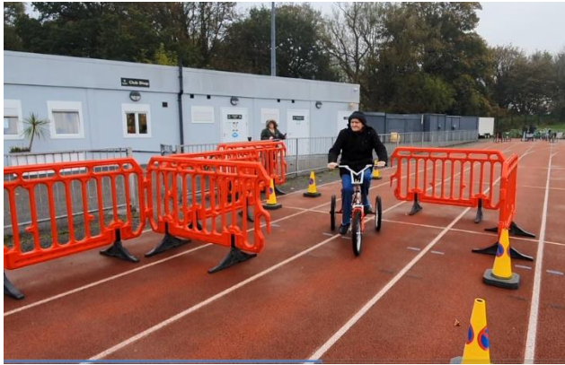
3.5m spacing of chicanes on 3m path. Picture shows tricycle.
