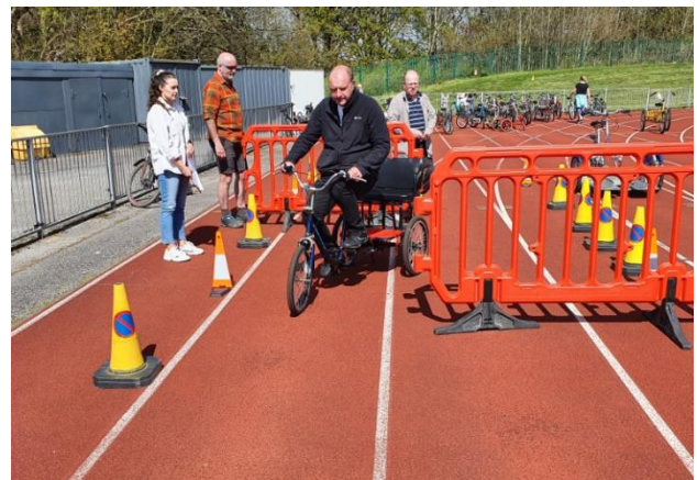
3.5m spacing chicanes on a 3m path with 0.3m overlap to reduce gap to 1.2m. Picture shows tricycle tandem.
