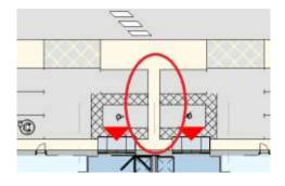
2) There is no pedestrian route past Unit 3E and the footpath in front of Unit 5A has a pinch point (see plan below).
