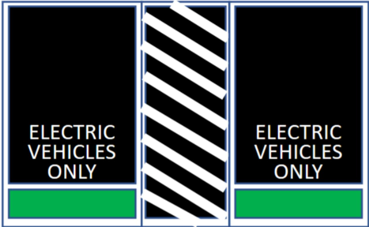
Figure 16 – Approved bay markings for electric vehicles <sup>36</sup>
