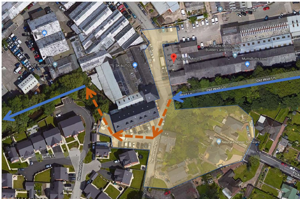
Figure F.13: Queens Road; Overhead view showing overland flow path in red.
