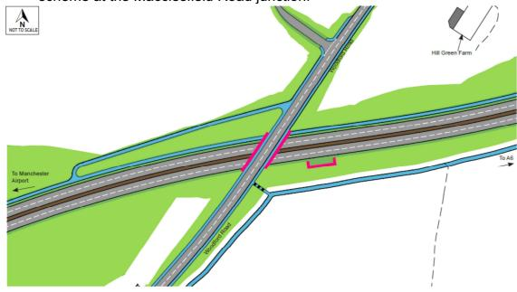
Option 2: Woodford Road connects to the scheme via two traffic lights controlled, staggered T-junctions.
